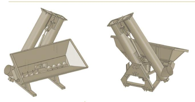
THE 6 METER - FEED HOPPER For side tipping.
